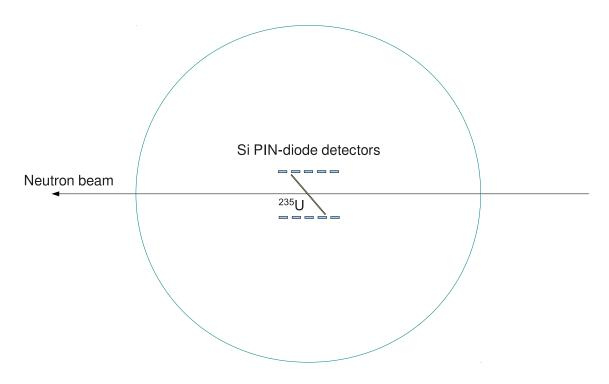
Fission fragments were detected by 5 pairs of Hamamatsu Si PIN diodes. Alpha resolution was 18 keV for 5475 keV line of <sup>241</sup>Am, timing res<sup>n</sup> was 100 ps.
